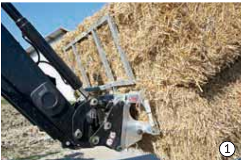
»Open View« pallet fork with guard rail
