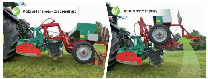
The hydraulic »Multi« adapter combines existing soil cultivation attachments such as rotary harrows, spike drums and short cultivators with seed drills and precision sowing machines of any attachment category.
