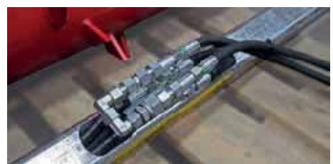
Illustration: Hoses are routed internally, sturdy support pipes
