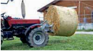
Illustration with round bale tines for transporting bales
