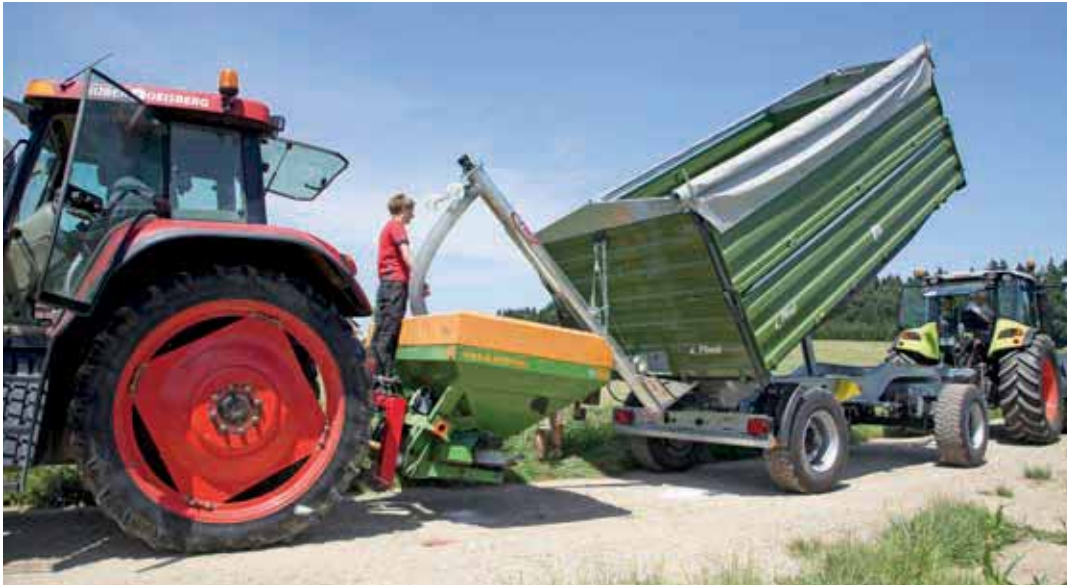
Fastening is extremely easy. The connecting piece is simply fixed in place on the side.
