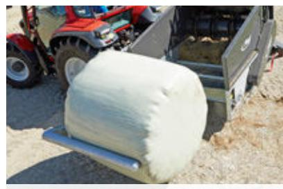
Hydraulically adjustable gripping arm
