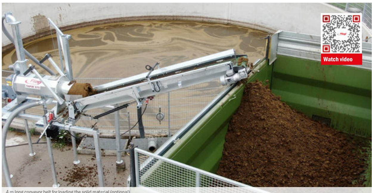
4 m long conveyor belt for loading the solid material (optional)
