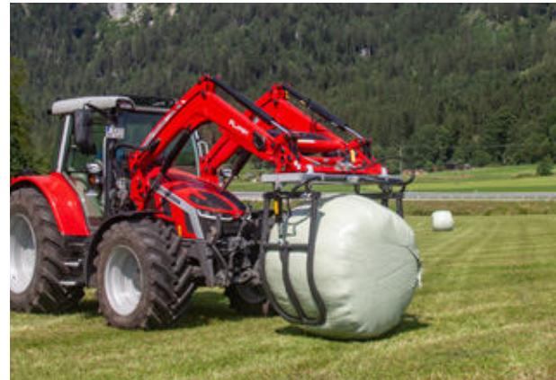
Grips bales securely, without causing damage
