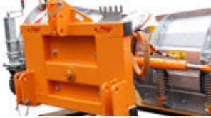
Innovative three-point headstock compensates for uneven ground
