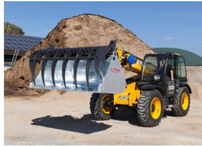
Tines made from highly wear-resistant steel HB 500 (thickness 20 mm)
