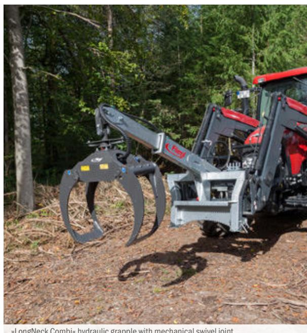
»LongNeck Combi« hydraulic grapple with mechanical swivel joint
