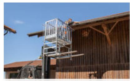
Attached to forklift with chain guard
