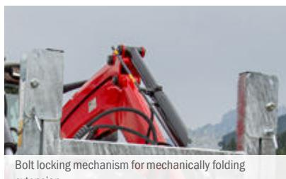
Bolt locking mechanism for mechanically folding extension
