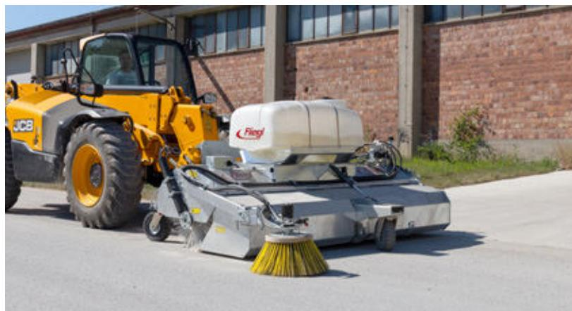
Infinitely adjustable sweeper roller – usable up to the maximum wear limit
