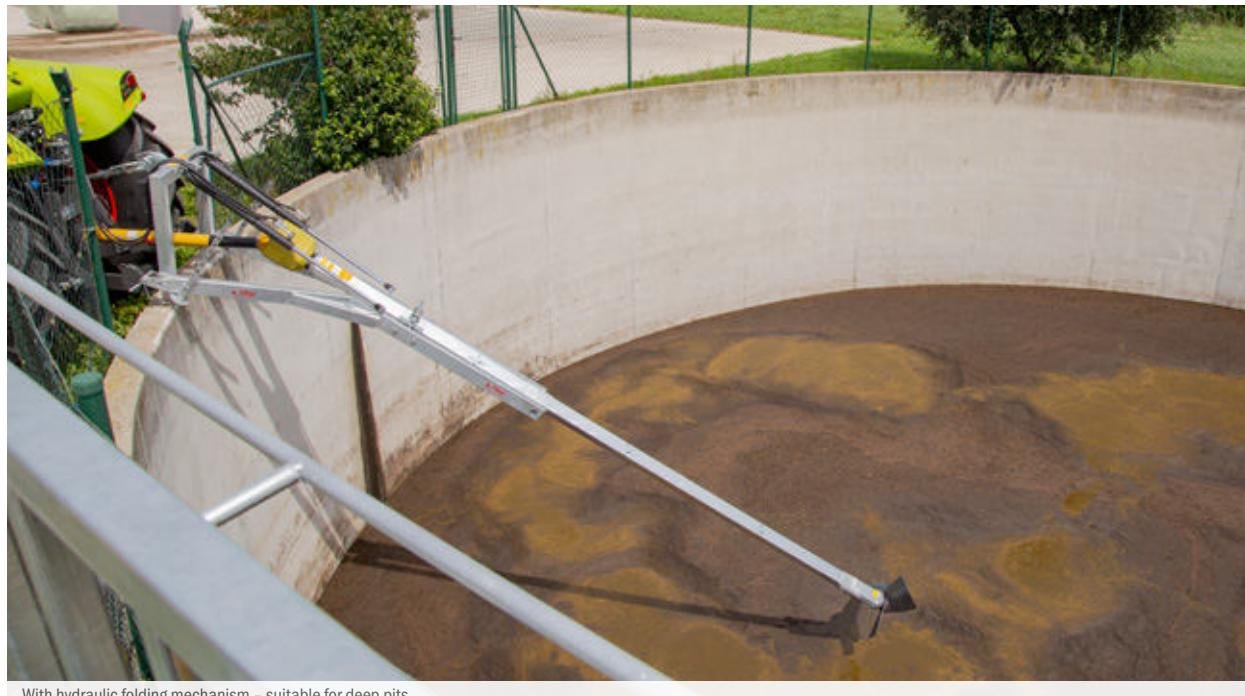
With hydraulic folding mechanism – suitable for deep pits
