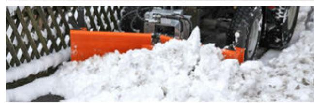
2 hydraulically pivoting wings with separate control
