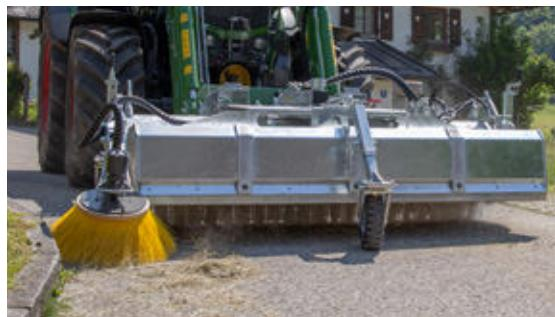
Shown here in free sweeping mode (enables sweeping with dirt collecting pan open by operating a shut-off valve)
