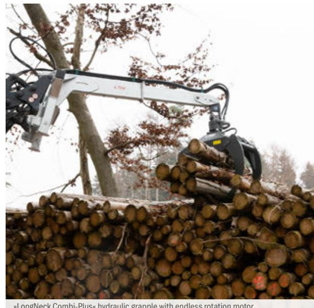
»LongNeck Combi-Plus« hydraulic grapple with endless rotation motor
