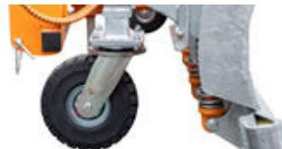
Heavy-duty support wheels with super-elastic solid rubber tyres: Ø 306 mm, width 105 mm, ball-bearing mounted, wear-resistant tread, heavy-duty slewing ring design, adjustable spindle
