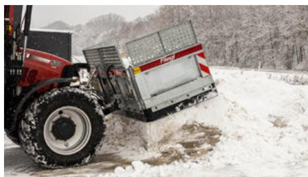
Clearing width infinitely adjustable via the 2 side wings, attachable grid (optional)
