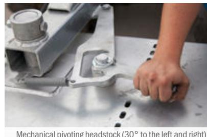
Mechanical pivoting headstock (30° to the left and right)
