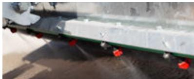
Spraying system – the splash guard nozzles are protected on the housing and spray the water close to the brush and prevent dust formation
