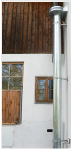
Installation example: inclined screw conveyor with head distributor on a silo
