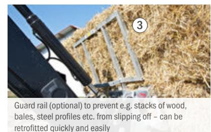
Guard rail (optional) to prevent e.g. stacks of wood, bales, steel profiles etc. from slipping off – can be retrofitted quickly and easily
