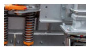
Spring-loaded overload protection ensures damage-free operation
