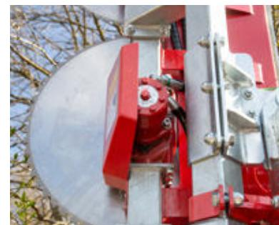
Saw blades powered via oil motors
