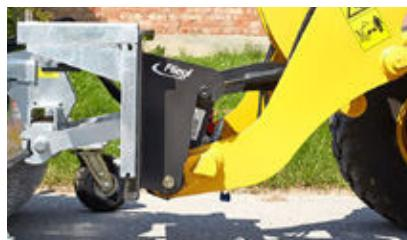
Wheel loader mounting with pendular compensation
