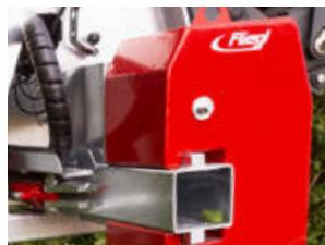
Lateral counterweight for minimal load on carrier vehicle linkages.
