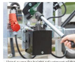
Hand pump for height adjustment of the conveyor belt
