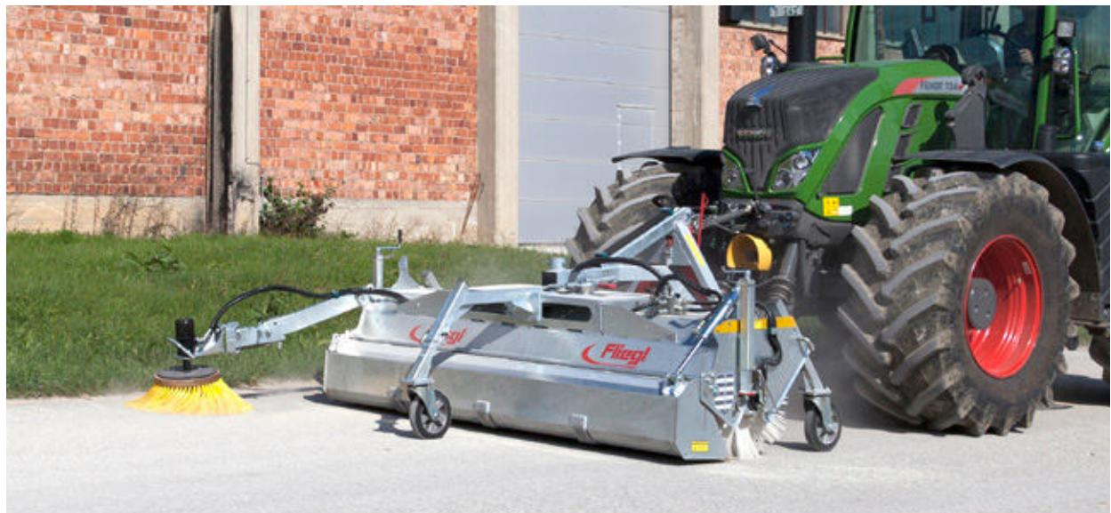
With three-point hitch, hydraulic dirt collecting pan, side brushes and support wheels
