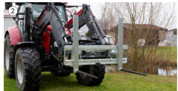
Adjustable mounting for round bale tines M28 x 1.5 mm
