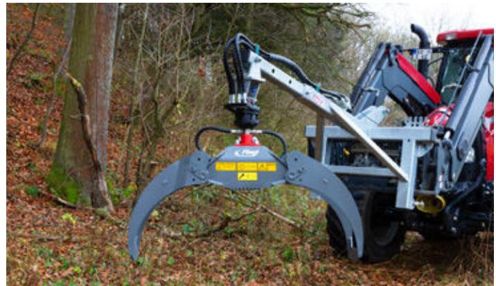
Loading gripper with load hook extension, rotary motor, Euronorm and three-point linkage
