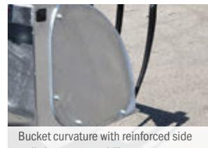
Bucket curvature with reinforced side walls increases stability
