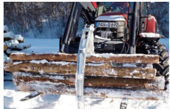
Hydraulic grab arm attached to »Open view« combi pallet fork
