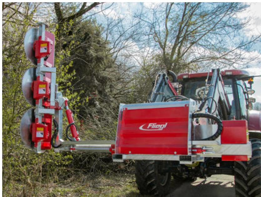
Flat, specially shaped cutting head for optimum visibility – ideal for cutting shrubs and coarse undergrowth.
