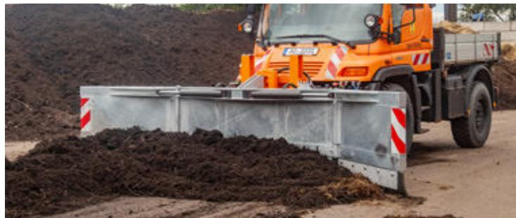
With rubber strips, durable thanks to moulded steel cables
