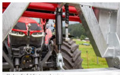
Hydraulic folding mechanism
