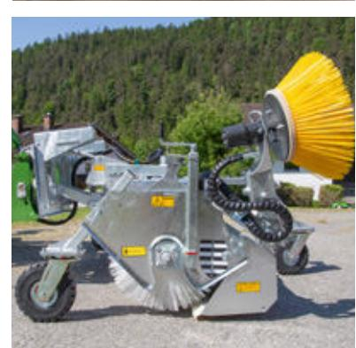
Sweeper roller is infinitely adjustable via a spindle and can be used up to the maximum wear limit
