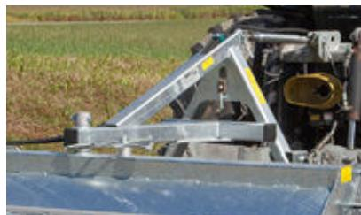
Three-point headstock for front and rear attachment
