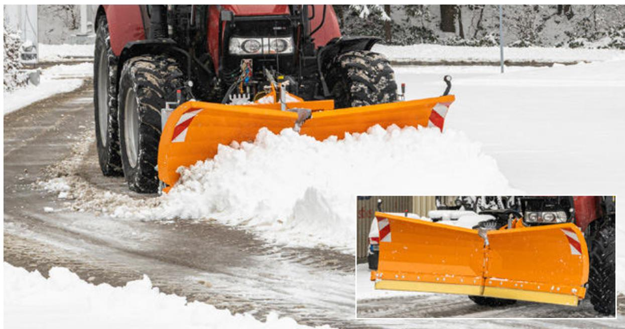
Two hydraulically swivelling wings can be controlled independently to select specific angle, plough or V settings
