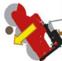
**Note:** Always cut thick branches from top to bottom to avoid jamming the saw blades!
