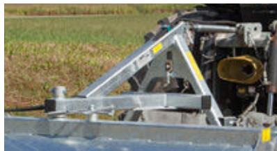
Three-point headstock for front and rear attachment
