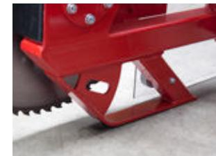
Guard rail prevents bottom saw blade from touching the ground.
